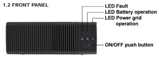
If the power supply cord is connected, press ON button and the PG 500 will work either in 230 V mode or in a battery mode, depending on whether the power supply is available. One more pressing the button will turn of the inverter control but the battery charging is maintained (supposed the incoming 230 V power is available).
